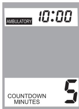
\* The screen will display X countdown minutes to indicate the time to the next automatic measurement.
