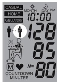
When measurements have been carried out for the full 7 days, the doctor symbol will flash on the screen.
