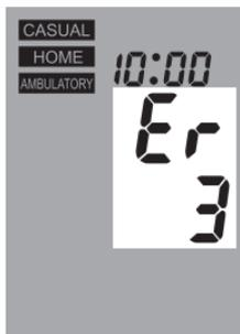
➔ **A repeat measurement is performed automatically if an error occurs.**
